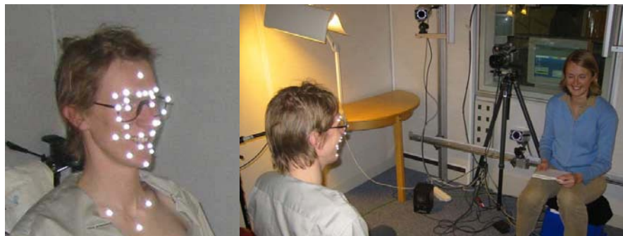
Fig. 3. Data collection setup with video and IR-cameras, microphone and a screen for prompts (right) and test subject with the IR-reflecting markers glued to the face (left)
