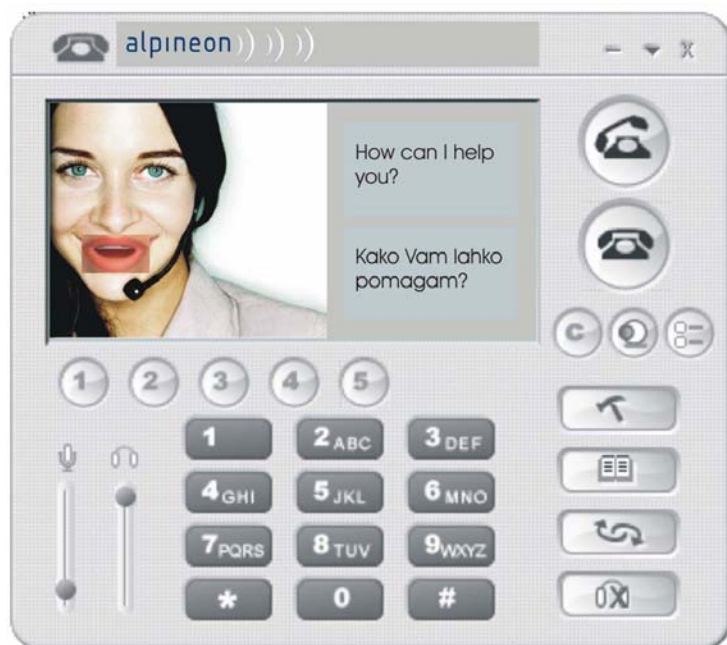
Fig. 2. Screenshot of the VideoTRAN VoIP software client. To the right of the window with the video image, utterances in both the source language (recognized utterances) and the target language (translated utterances) are displayed.
